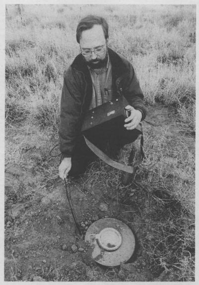
MINE SNIFFER — Phil Rodacy (1552) demonstrates a mock chemical sensing detector on an antitank mine in the makeshift minefield in Tech Area 3. The final field-ready sensor probably will look similar to the mock detector and will be easy to use. (Photo by Randy Montoya)
